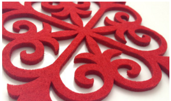
Clean and perfectly sealed laser cut edges of textiles
