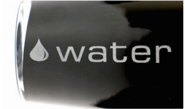
Laser engraved drinking glass with rotary device
